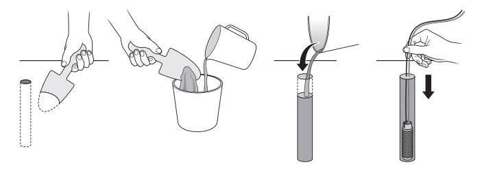
4. Place sensor in vertical position (do not tilt more than  $45^{\circ}$ ) at bottom of hole.
