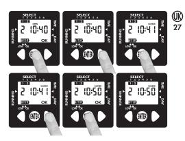
WATERING PROGRAM 2 IS SET TO START AT 10:40 AND END (CLOSED) AT 10:50
